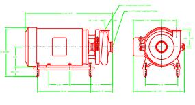
MOTOR SPECIFIC ATIONS: BALDOR - TEFC 3 PHASE 60 HZ 230/460 VOLTS 10 HP @ 3500 RPM 213JM FRAME
