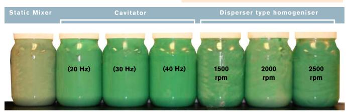
APV Cavitator in comparison with static mixer and homogenizer. Mixing pigment and other post additional ingredients with high viscous base cream liquids.
