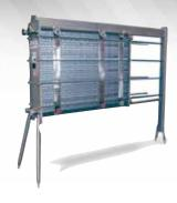
frame sizes holding up to a maximum of 500 plates (0.02" (0.6 mm) thick) are available with a port diameter of 2.5" (64 mm) making the Vega frames capable of processing up to 250 gal/min or 57 m³/h of product. Plates are available in a wide thickness range of .02" to .03" (0.5 to 0.8 mm) making them adaptable to a large range of process design pressures.
