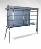
frame sizes holding up to a maximum of 500 plates (0.02" (0.6 mm) thick) are available with a port diameter of 2.5" (64 mm) making the Vega frames capable of processing up to 250 gal/min or 57 m³/h of product. Plates are available in a wide thickness range of .02" to .03" (0.5 to 0.8 mm) making them adaptable to a large range of process design pressures.
