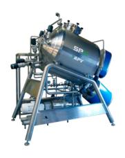
**Principle:** The Flex-Mix processor tank is filled with water. The temperature is dependent on the fat/stabilizer requirement.
