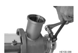
Figure 38 - Installation of Hinged Clamp
