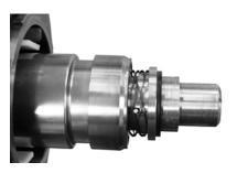
Figure 70 - Double Mechanical Seal Installed
