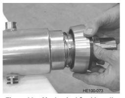
Figure 33 - Mechanical Seal Installation
