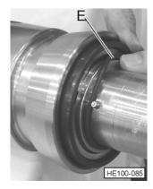
Figure 57 - Install Keeper O-ring
