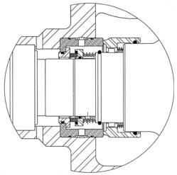
Figure 5 - Double Mechanical Seal
