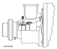
Figure 3 - Double Mechanical Seal
