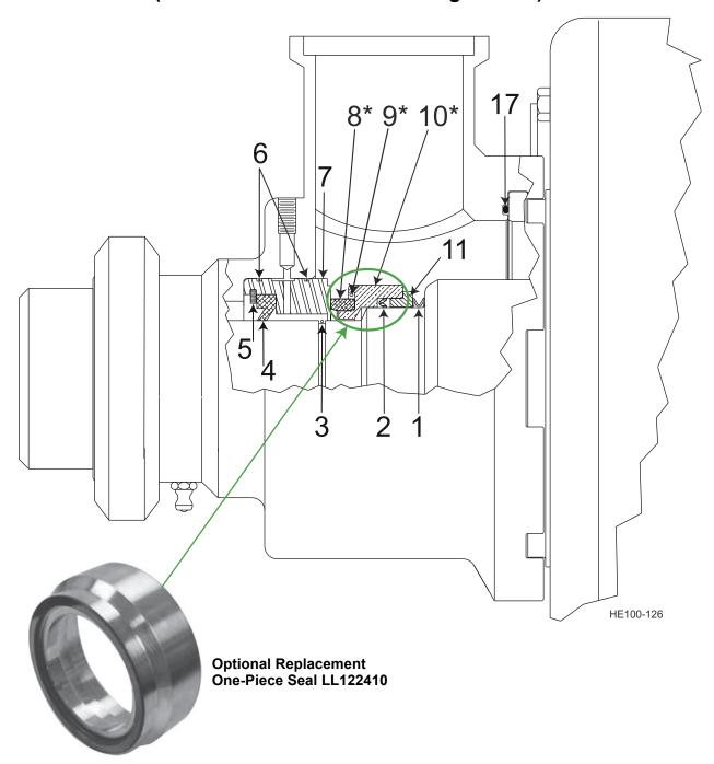
This is the standard rotating single mechanical seal for all Votator IIs manufactured between 1997 and 2004. The seal body is positioned on the 2.25-inch diameter stub ends of the mutator. This seal can be retrofitted to a one piece design by replacing items 8, 9, and 10 with a chrome oxide one piece body, p/n LL122410, and running it against a ceramic head insert, part number LL928508.
