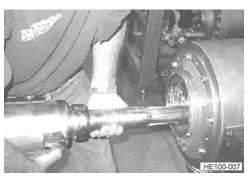
Figure 30 - Removal of Shaft Drive End
