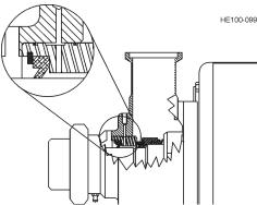
Figure 2 - Single Mechanical Seal
