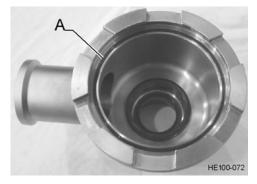
Figure 35 - Opposite Drive End Head O-ring
