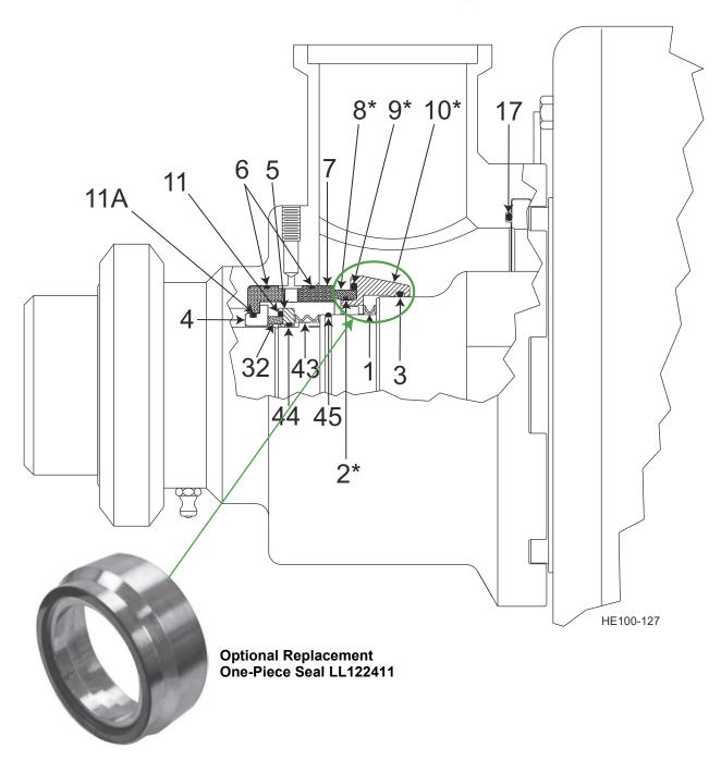
This is the standard double mechanical seal for all Votator IIs manufactured between 2000 and 2004. The primary seal body is positioned on the 2.75-inch diameter stub ends of the mutator and the secondary seal body (Item 5) is positioned on the 2.25-inch diameter stub ends. The two-piece primary seal body can be retrofitted to a one-piece design by replacing items 2, 8, 9, and 10 with a chrome oxide seal body, p/n LL122411 running against a ceramic head insert, p/n LL934873.
