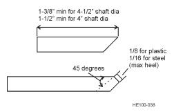
Figure 25 - Blade Wear and Sharpening
