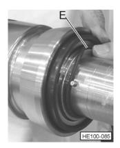
Figure 69 - Install Keeper O-ring
