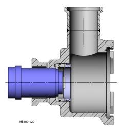
Figure 59 - Gland and Seat Removal
