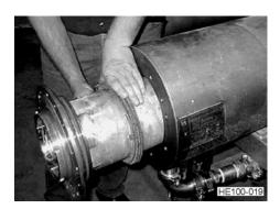
Figure 40 - Tube Removal
