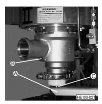
Figure 42 - Location Of Hydraulic Arm For Removal
