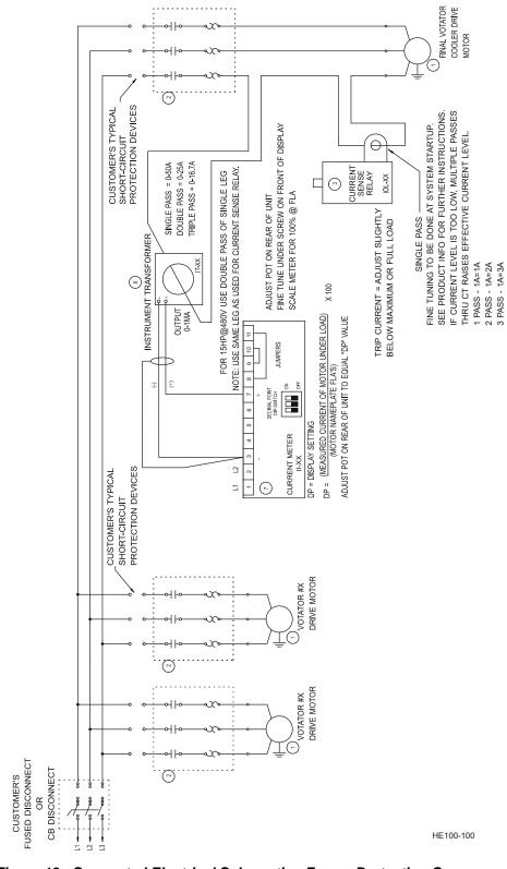
Figure 13 - Suggested Electrical Schematic - Freeze Protection Components
