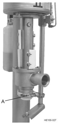
Figure 74 - Remove Head Clamp
