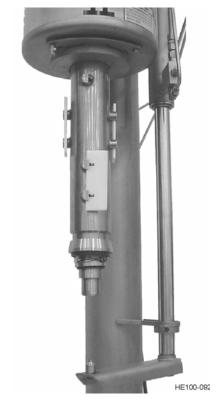
Figure 75 - Shaft With Head Removed
