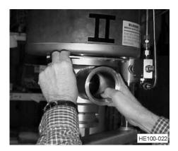
Figure 48 - Close Locking Latch
