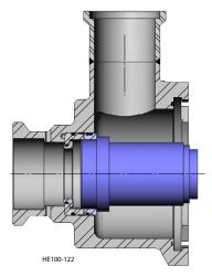
Figure 62 - Seal Installation
