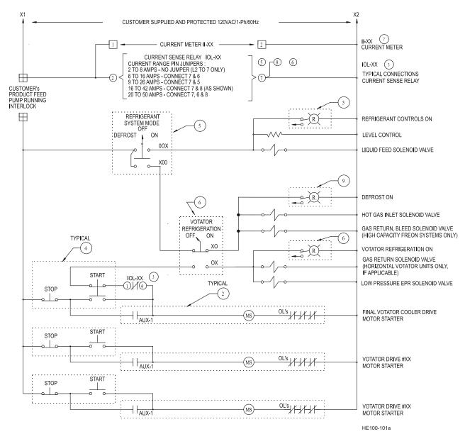
Figure 14 - Suggested Electrical Schematic - Gravity Refrigeration with Level Master Control (LMC)
