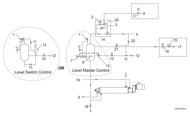
Figure 11 - Suggested Media Piping, Gravity Refrigeration - HORIZONTAL
