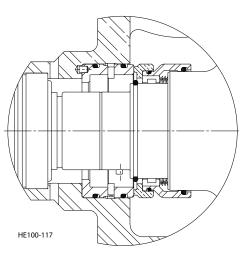
Figure 6 - 2012 Single Mechanical Seal
