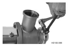
Figure 26 - Removal of Hinged Clamp
