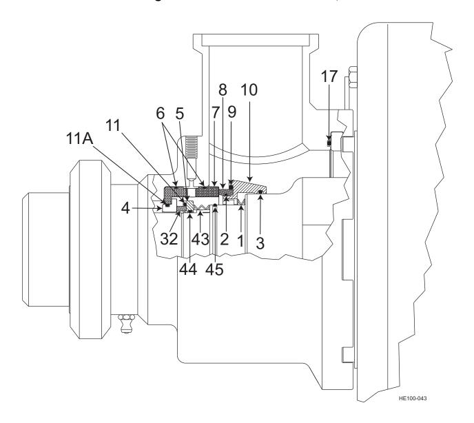
This is the standard mechanical seal for most Votator IIs manufactured between 2000 and 2004. The primary seal body is positioned on the 2.75-inch stub ends on the mutator. If the unit has a double mechanical seal, including secondary items 4, 5, 11, 11A, 32, 43, and 44, the secondary seal body (Item 5) is positioned on the 2.25-inch stub ends of the mutator.
