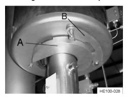
Figure 73 - Installed Shaft Clamp
