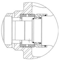
Figure 4 - Single Mechanical Seal
