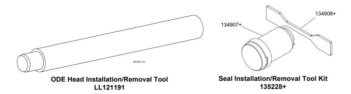
Use ODE Head Installation Tool LL121191 to protect head insert when installing or removing the opposite drive end product head. Seal installation tool kit 135228+ can be used for inserting and removing the gland and seal. The small end is used for secondary seal installation and removal and removal of the gland and seat. The large end is used for gland and seal seat installation.
