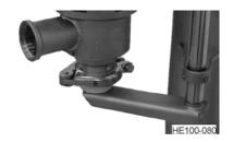
Figure 45 - Head Installed on Pin
