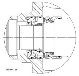
Figure 7 - 2012 Double Mechanical Seal (shown with Narrow-Face Rotary)
