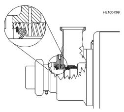
Figure 54 - Lip Seal Orientation
