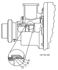
Figure 56 - Orientation of Seal Components
