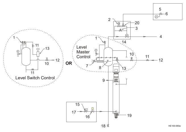
Figure 12 - Suggested Media Piping, Gravity Refrigeration - VERTICAL
