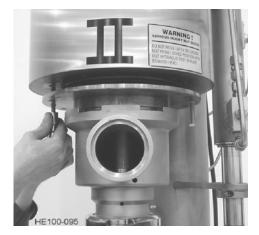
Figure 51 - Insert Jack Screws
