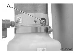
Figure 21 - Pressure Adjustment Screw
