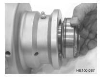
Figure 23 - Lubrication Ring Orientation
