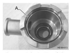
Figure 32 - Drive End Head O-ring
