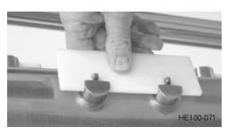
Figure 24 - Scraper Blade Removal
