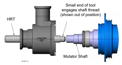
Figure 28 - Use of Head Removal Tool (HRT)
