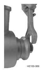
Figure 27 - Removal of Shaft Locknut
