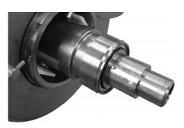
Figure 68 - Install Seal Body
