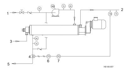
Figure 9 - Suggested Media Piping, Water or Liquid
